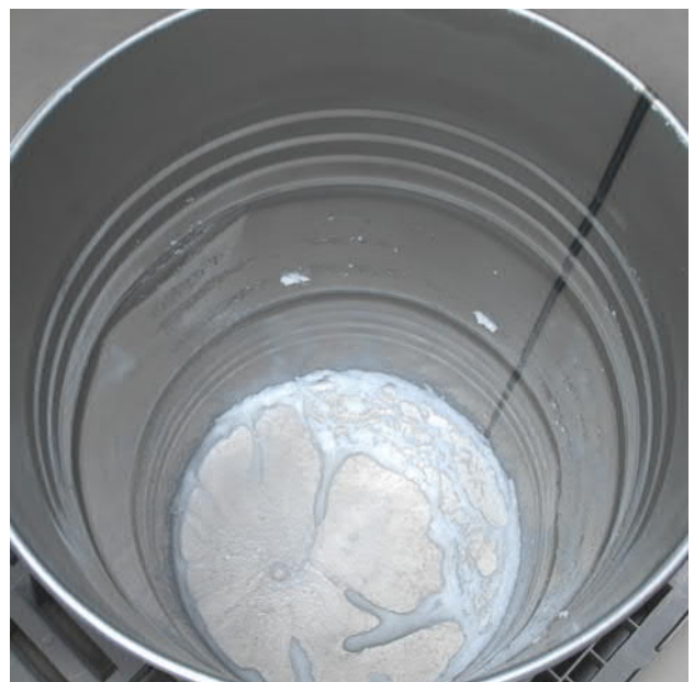
VISCOFLUX mobile S achieves minimal residual quantities, even for drums with standard transport dents.
